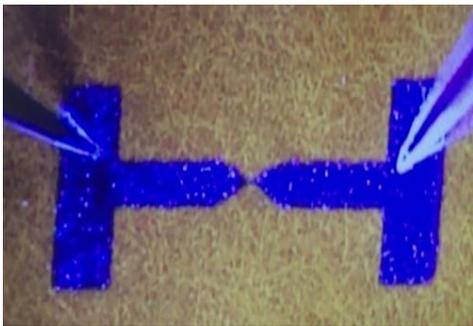
Fig. 2. Optical image of the source and drain layers printed on Kapton substrate using silver ink.
